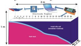
Figure 2.Layout measurement that include translational slide, rotational slide,debris avalance, debris flow, lateral spread and slump earthflow
