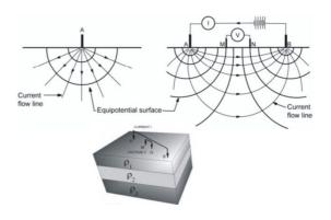
Fig.1 Electrode arrangement for apparent resistivity measurements(Kirsch, 2009)
